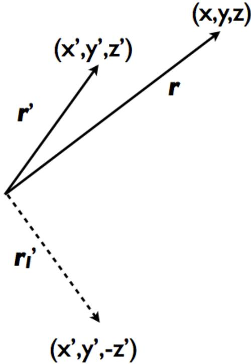
Figure 33: Relationship between the vectors  $\mathbf{r}$ ,  $\mathbf{r}'$ , and  $\mathbf{r}'_I$  for the Dirichlet Green's function for an infinite plane. These three vectors label the field location, source location, and image charge location, respectively.
