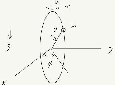
$$\phi = \omega t \quad (\text{peculiar}) \rightarrow \dot{\phi} = \omega$$
