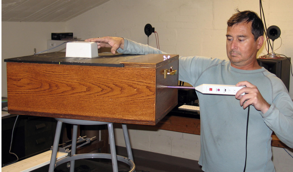
Figure 1. Acoustics box (as shown or use an available wooden cube) to simulate the acoustics of a room (built by Arnold Fernandez). The small speaker at the top excites box resonances with a sine sweep or white noise. The microphone inserted on the right records the resonances.
