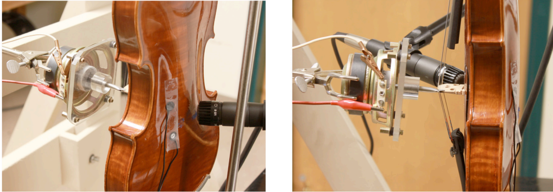
Figure 5: Mounting of the violin for recording the response from the back plate (left) and front plate (right). The driving rod of the vibrator is fastened off-center to the bridge of the violin with a clip. Note the microphone positions in both pictures. (A piezoelectric transducer can be taped to the back (or front) to complement the microphone measurements.)
