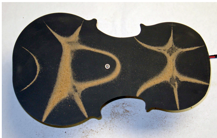
Figure 1: A Chladni figure from a metal sheet simulating the back plate of a violin. The resonance frequency for this pattern is 428 Hz.
